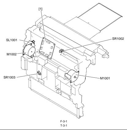
JAM code/E code Ref. Parts number Name Duplex controller PCB FM2-4515 [1] E052 M1001 FK2-1114 Feed motor M1002 Reversal motor FK2-1114 SL1001 Duplex flapper solenoid FL2-3744 SR1002 Duplex paper sensor 1 (upper) WG8-5696 0120, 0221 SR1003 Duplex paper sensor 2 (lower) WG8-5696 0124, 0228
